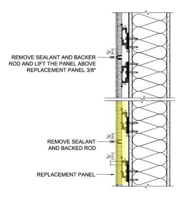
Step 1: Move Panel Above Panel to be Replaced
